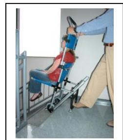
3. Push the Evacuation chair down the first step carefully until the track is sitting level on the steps; ensure you are holding the Evacuation Chair securely. T
